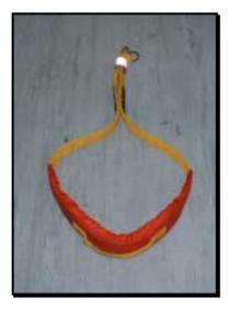
**Figure 7.21 SAR Rescue Strop** (photograph courtesy of CHC Scotia)
