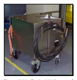
Figure 7.23 Typical Helicopter Start Facility
