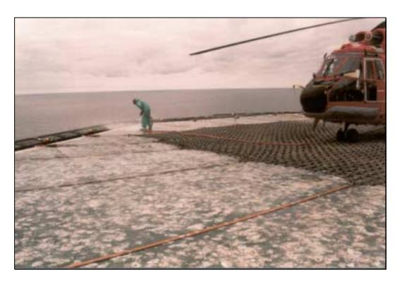
Figure 10.2 An Example of the Effects of Guano Infestations on a Helideck Surface
