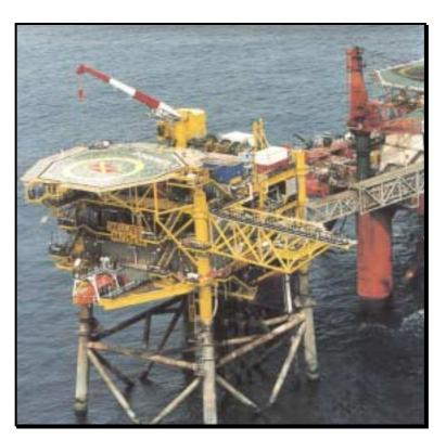
Figure 9.3 Example of a Temporary Combined Operations Arrangement with a NUI and Accommodation Vessel Bridge-linked
