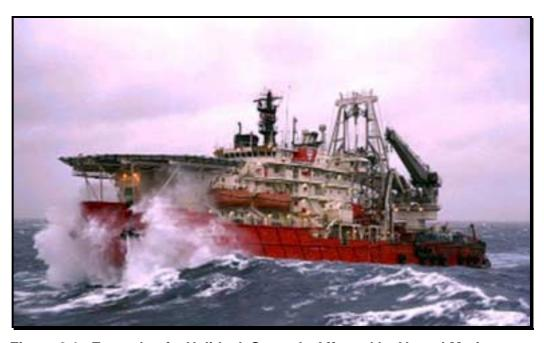
Figure 8.1 Example of a Helideck Severely Affected by Vessel Motions
